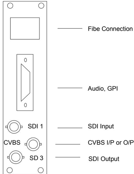
Note: It is also possible to use the rear panel designed for the V6351 and V6751 series of audio embedders and de-embedders (V16VR3R), but then there is not a dedicated BNC for the CVBS. In that case the CVBS connection must be made through the HDD audio/GPI connector. See section 3.3.3.
