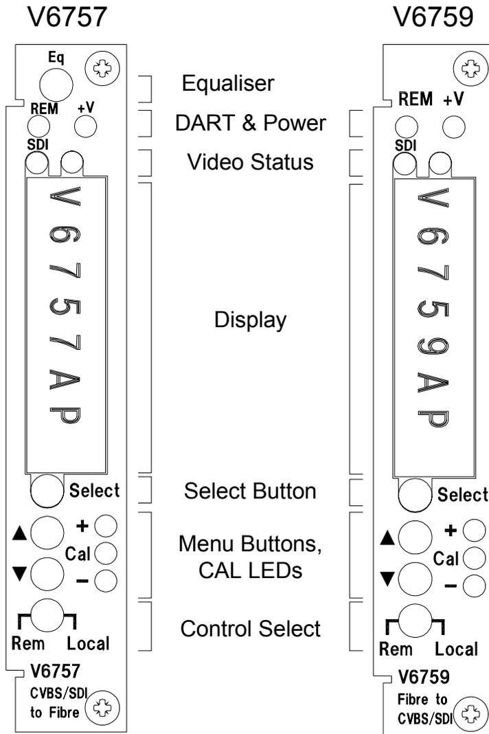
The front panel on the V6757 and V6759 are a considerable advance on what is usually available on single module interface equipment. It provides the user with total control and monitoring of the unit without the need to consult manuals and read unlabelled indications. While this kind of control is generally available with a remote control system, as it is over DART, it is unusual to have this level of access locally.
