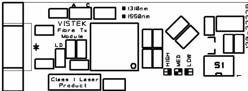
It is important that the output power of the Laser transmitter is set so as to be suitable for the receiver. Receivers have a maximum input power level, often specified as the ‘Saturation Power’, which should not be exceeded for reliable transmission. For short haul it is possible to use an optical attenuator to avoid saturation in the receiver.
