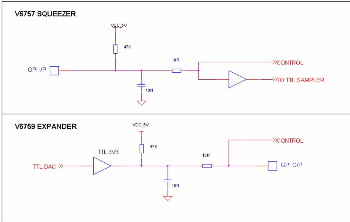
On the V6757 Squeezer the GPI input pin feeds both the standard digital GPIs and the sampler on the sub-module. If they are being used for an real time varying signal over the link, then the digital GPIs should be disabled on the `CONFIG: GPI` menu. All three GPIs can be used independently. There is no reason why one can't be used for analogue while the other two are for digital.
